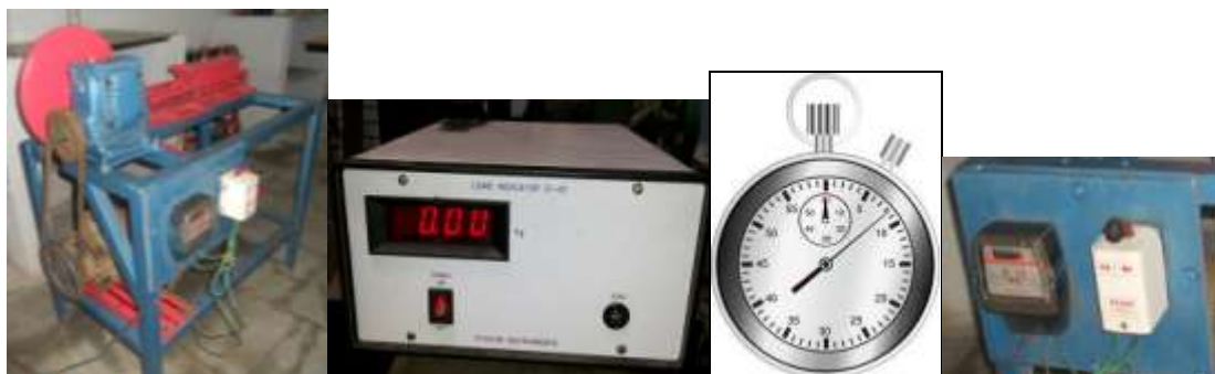
Fig. 1: Experimental Set-up along with measuring devices a) Load cell b) Stop watch c) Energy meter
